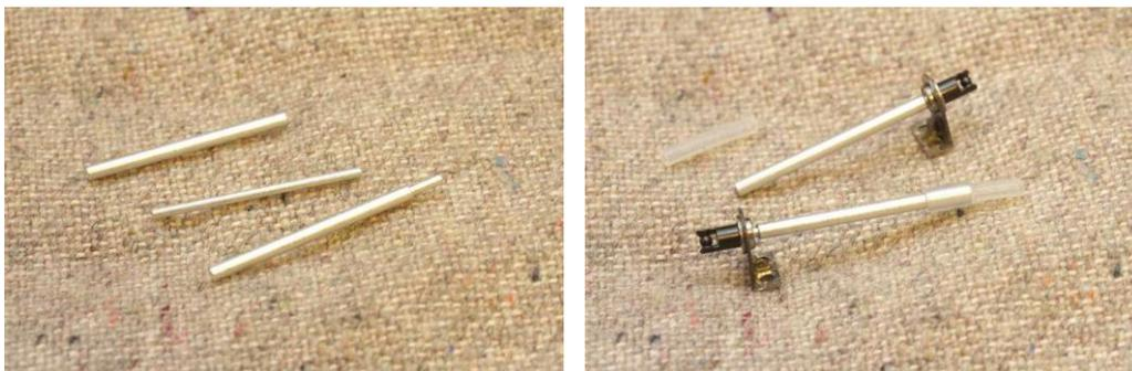
The sections of tube can then be joined, with 7mm of the inner tube protruding. I used Loctite 480, but an epoxy would work as well. Apply the adhesive to the outside of the thin tube as you feed it in – the inside of the larger bore must be clear of any adhesive. Once the adhesive has cured add the drive bracket, drive coupling and a 15mm length of neoprene tubing to complete the assemblies.
