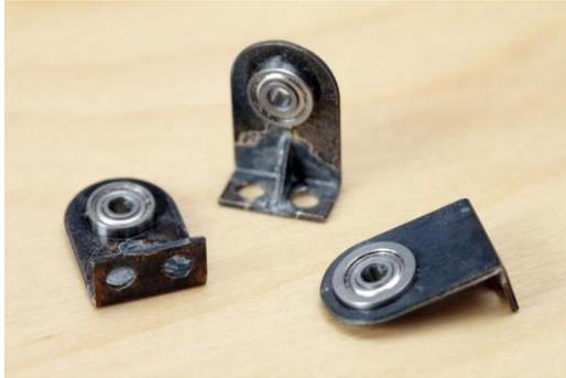
The bearing brackets also need folding, the reinforcing ribs added and can be blackened. The bearings are then fitted with Loctite 603. If you take care to make the items up like this (look at the bearing orientation) then the dimensions quoted later in this note will work for you.
