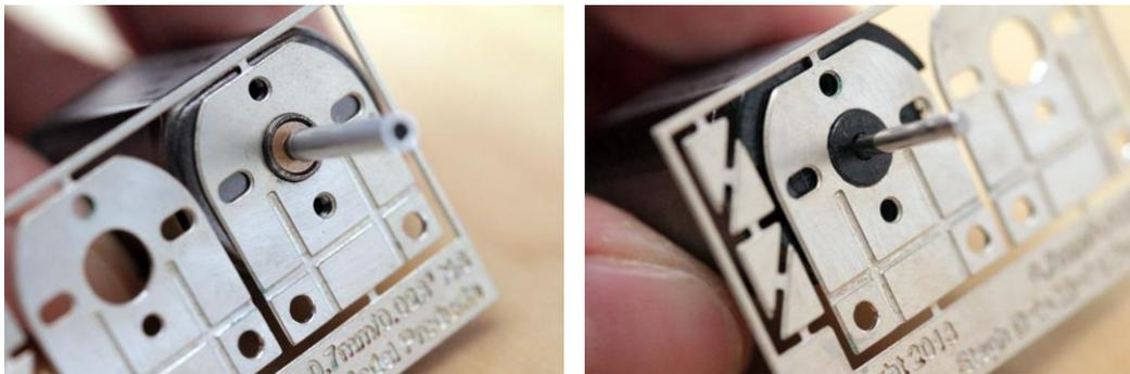
This is the fitting for the motor front (left) and rear (right). Some care will be needed for the fitting on to the back boss as this must be tight to prevent the motor vibrating.
