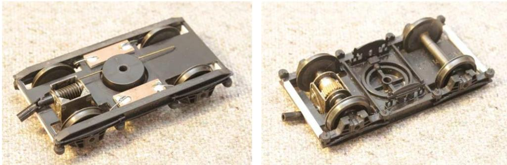
First step is to build the gearboxes and assemble them into the bogies. The bogies shown here are by Easybuild, but any bogie could be used. Two things are worth noting; 1, it helps if the torque reaction arm is long and straight, and; 2, there may be a need to put a notch or step in the inner end beam to clear the drive shaft: For first-generation BR DMUs this is prototypical!
